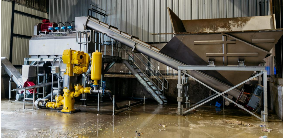
Figure 6 – Food waste de-packaging line receiving food waste at an anaerobic digestion site
